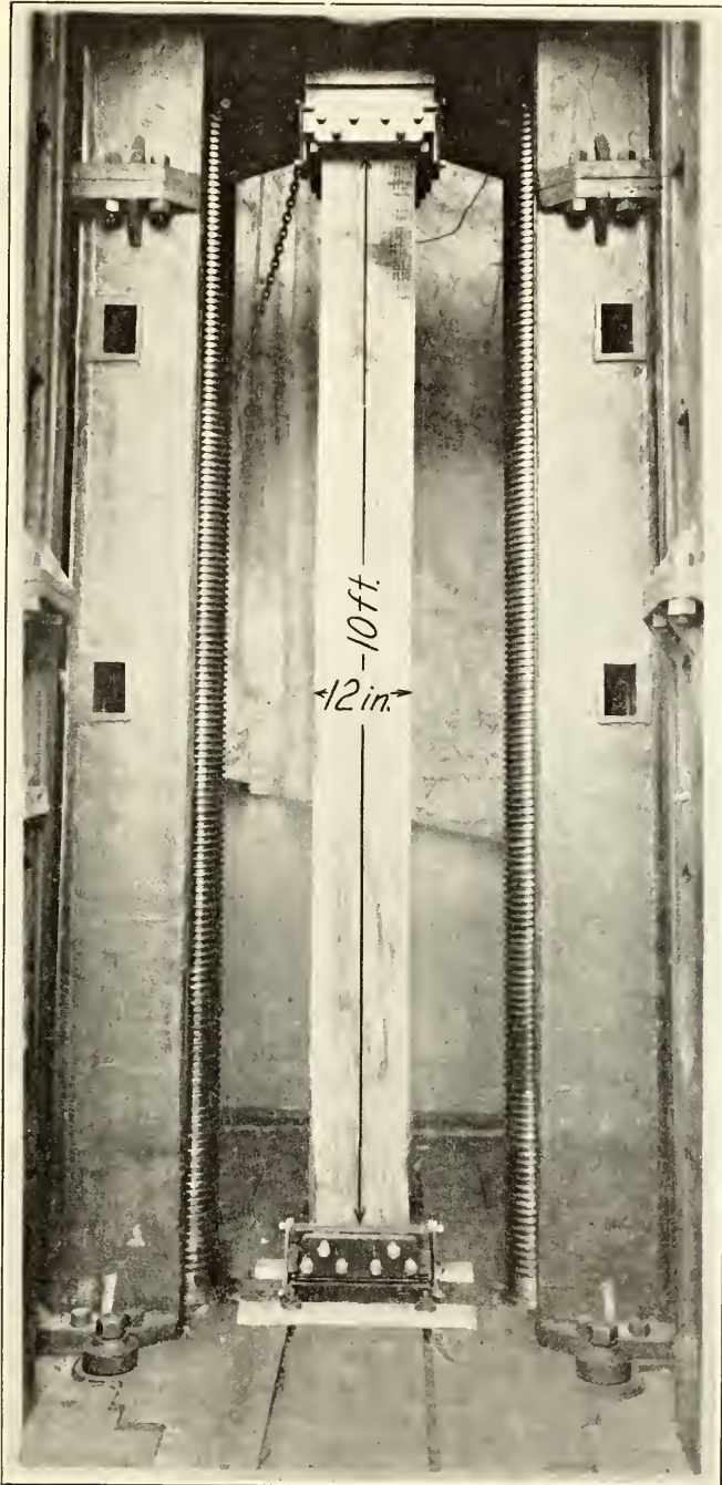
An intermediate column in the Forest Products Laboratory 1,000,000-pound timber-testing machine
